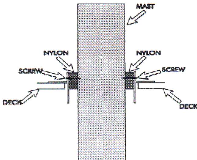
5. When the mast is straight, it is pinned down with a piece of nylon which is screwed through the mast collar so the mast is centered in the boat.
